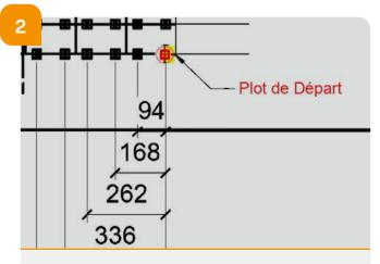
→ Check the positioning of the pedestral of reference using the EXECUTION DRAWING.
