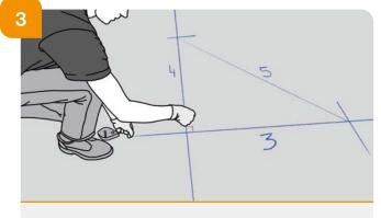
→ Square the installation area using a chalk line with the 3-4-5 method.
