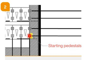
→ Check the positioning of the pedestal of reference using the EXECUTION DRAWING.
