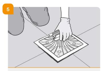
→ Ensure the positioning of the **SOPRASOLAR® FIX EVO** pedestals. The center of each pedestal is marked by the intersection of the drawn lines.
