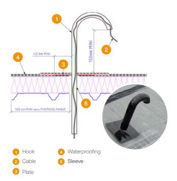
Cross-section view for grounding connection
