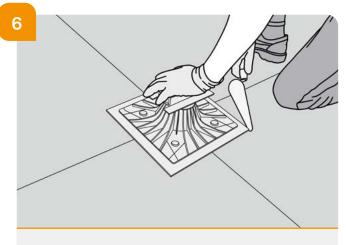
→ Mark the outline of the pedestal using a trowel to indicate its position on the roof.
