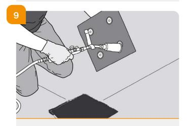
→ Melt the thermofusible film with the torch, then heat the underside of the base.
