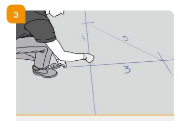
→ Position the SOPRASOLAR® FIX EVO pedestals. The center of each pedestal is marked by the intersection of the drawn lines.
