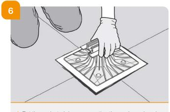
Put the pedestral down respecting the marks and apply pressure. You are at stage 0 5
