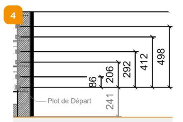
→ Mark the reference points using a chalk line, following the dimensions from the EXECUTION DRAWING.
