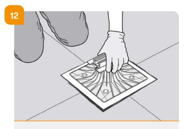
→ Apply the pedestal to the membrane and press down to confirm the weld.
