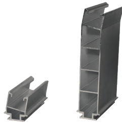
Low and high raisers For connecting Soprasolar® Fix Evo Tilt pedestals to photovoltaic modules while creating a 10° tilt angle. They must be used in combination with booster locking frames.
